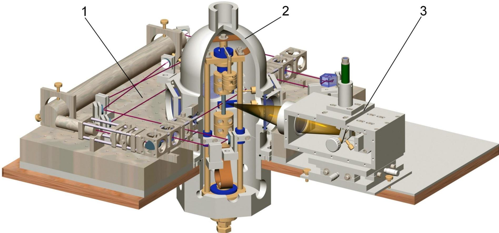
1 interferometer, 2 vessel, 3 pyrometer
