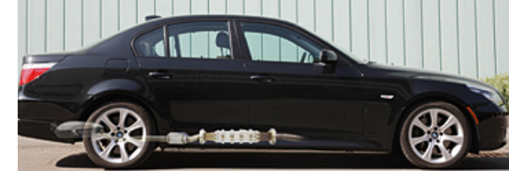
Schematic of a TEG incorporated with a special heat exchanger installed in an exhaust system. Courtesy of Dr. Bassem Ramadan.
